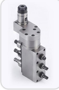
360° Angle rotary tool holder Speed ratio:1/1 Max speed:6000RPM Angle range:0°~360° Collet type: Main spindle ER16 Sub spindle ER11
