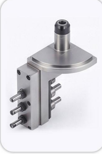
90° Angle rotary tool holder Speed ratio:1/1 Max speed:6000RPM Angle range:0°~90° Collet type: Main spindle ER16 Sub spindle ER11
